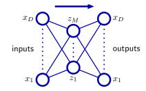
By setting the number of hidden nodes to be less than the number of inputs/outputs, we force the network to compress the data.
